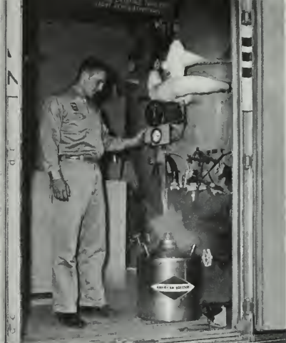
Recharging a technician's refrigerator with liquid nitrogen at a distribution point. The small refrigerator holds about 500 ampules of semen and enough liquid nitrogen for 2 weeks' storage. Frozen semen permits more efficient utilization of semen.
